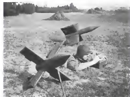
COBRA anti-tank guided missile package on soldier operates manual control box. Cobas are fitted with indigenous guidance system, control a shaped warhead over visual range.
